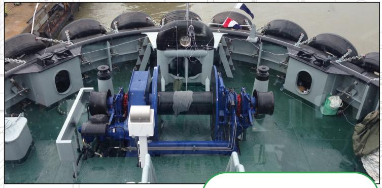
Windlasses with warping heads of cast steel hawsers tillage. Chain lifter of cast steel provides with clutch to allow independent operation of the warping heads, with independent brakes.
